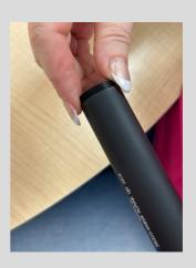
4. Identify blast baffle (first baffle towards mount). If stuck, do not use a screwdriver to remove.
