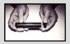
3. Sit muzzle the end of the suppressor on a flat surface, then remove the suppressor housing by lifting straight up to expose the baffle stack.
