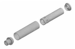
When replacing the M-Baffles into the central core, align the jets to all be lined up in arrow and keyed with the notches and tangs keyed together. The last baffle has no tangs because it seats up against the retainer. To assemble, follow these directions in reverse.
